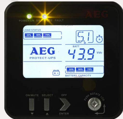
UPS switched to battery operation
