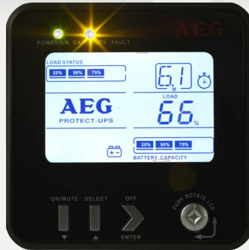
UPS switched to battery operation
