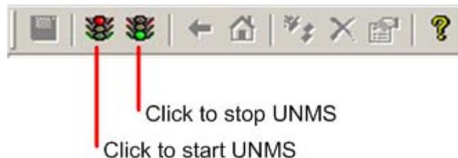
Restarting or stopping UNMS, or rebooting your UNMS server computer, is a severe action. When you restart the UNMS service, all sessions connected to your monitored devices are dropped. Any status and measurement data held from the monitored services are lost. All **Web Console** connections are unavailable until UNMS is restarted. For this reason, you should avoid restarting, stopping, or rebooting your UNMS server if at all possible.
