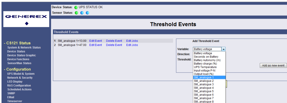
Figure 101: CS121-Configuration Threshold Events of analogue Inputs
