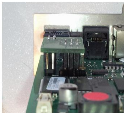
Figure 148: CS121 WDP piggyboard installed on a CS121 SC/BSC – view from left and behind
